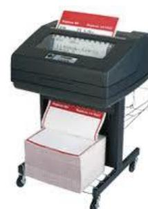
✎ This printer prints one line at a time, so it is called "line printers", in such a way that the printer's printing quality is not good, but its speed is much higher than that of dot matrix printers.
